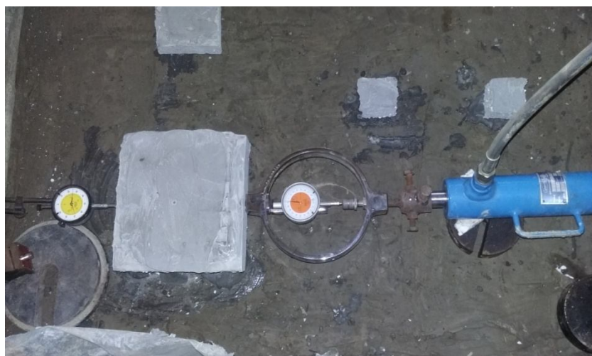
Experimental set up for Micropile lateral load capacity
