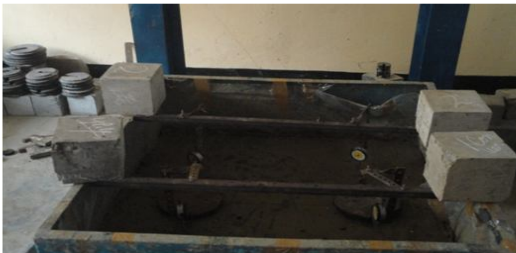
Experimental set up of Micropile-raft foundation
