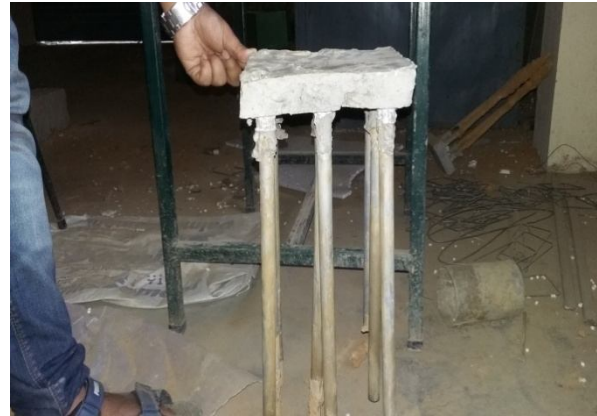
Micropile group bearing 9 number of pile Lateral load test
